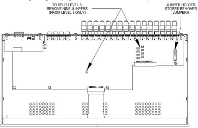
**NOTE:** Eight of the nine jumpers are grouped together. Do not forget to remove the ninth jumper that is located separately from the other eight.
