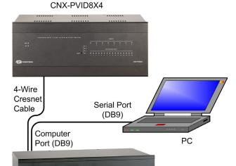
Typical Connection Diagram when Uploading
