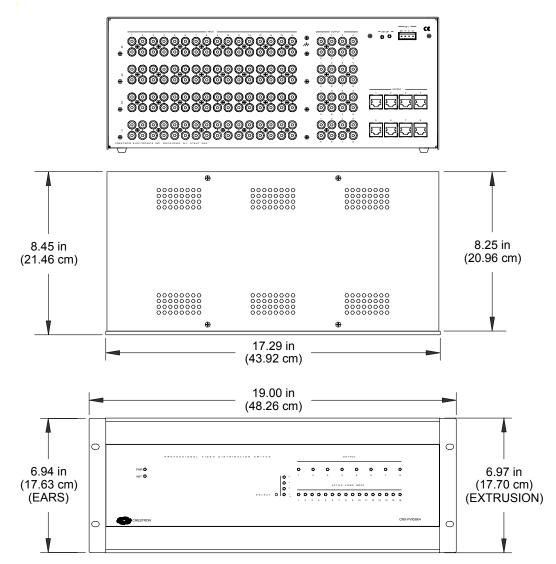
Two mounting ears are provided for rack mounting; four square rubber feet are provided for tabletop mounting or stacking. These feet are to be attached on the base of the unit for stability and to prevent slippage.
