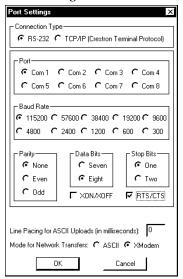
**NOTE:** The parameters shown in the illustration above are the port settings for a 2-Series control system. Consult the Operations Guide for the control system being used for exact parameter selection.
