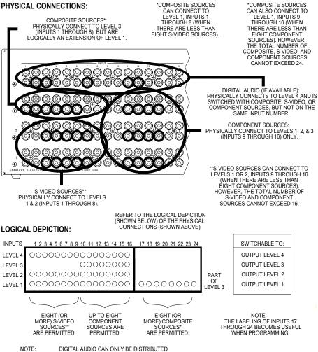
DIGITAL AUDIO CAN ONLY BE DISTRIBUTED FOR A TOTAL OF 16 SOURCES. IF DIGITAL AUDIO IS DISTRIBUTED WITH THE S-VIDEO DEVICE CONNECTED TO INPUT 1, INPUT 17 WOULD BE PROHIBITED FROM USING LEVEL 4 FOR DIGITAL AUDIO (AND VICE VERSA).
