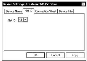
**NOTE:** SIMPL Windows automatically changes Net ID values of a device added to a program if a duplicate device or a device with the same default Net ID already exists in the program. Always ensure that the hardware and software settings of the Net ID match. For Net ID hardware setting details, refer to "Identity Code" on page 9.
