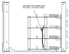
5. If the desired application requires removal of the jumpers, remove the nine jumpers from level 3 (top board) only, as shown in the diagram after this step. Otherwise, skip this step and step 6.
