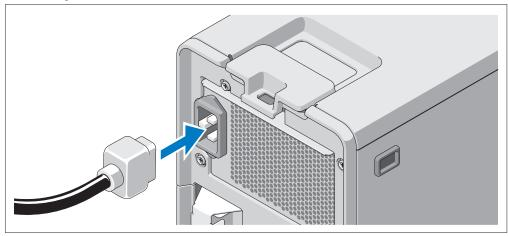
3 Connect the monitor power cable to the monitor (optional), and connect the system's power cable to the system.
