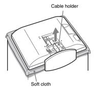
2 Remove the screws and detach the Table-Top Stand from the TV.
