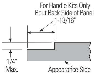
Rout the panel when installing a ZKHTR1 Custom Handle Kit or ZKHTRSS1, Tubular Stainless Steel Handle Kit.
