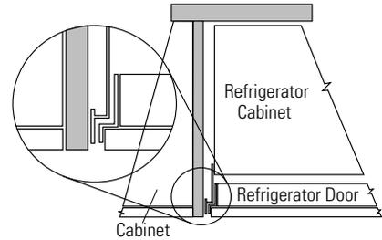
Note: 1/2" thick side panels shown. Side panels can be any thickness. Add side panel thickness to outside trim width (36" or 72" for two models) to calculate the rough-in dimension. The leading (front) edge must be finished to match surrounding cabinetry.
